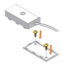
Go back up the ZLEAK on its support as indicated on the photo.
