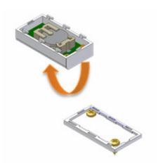
Press on the central leg of the support of battery to remove the battery.
