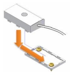
Proceed then to the installation of the sensor. With an adhesive, install the sensor on the zone to be watched.
