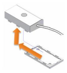
Locate the position of holes and drill the wall by taking into accounts your system of fixation (ankle + screw). Push ankles in the holes make previously. Position the support of the ZLEAK on the wall and screw saws them as on the photo.
