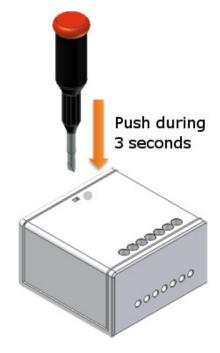
If the ZPILOT was not associated it begins flashing quickly during 20 seconds. The ZPILOT looks for a coordinator during this blinking.
