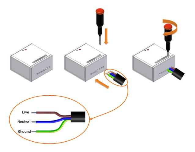
Connect the wire pilot on the ZPILOT.
